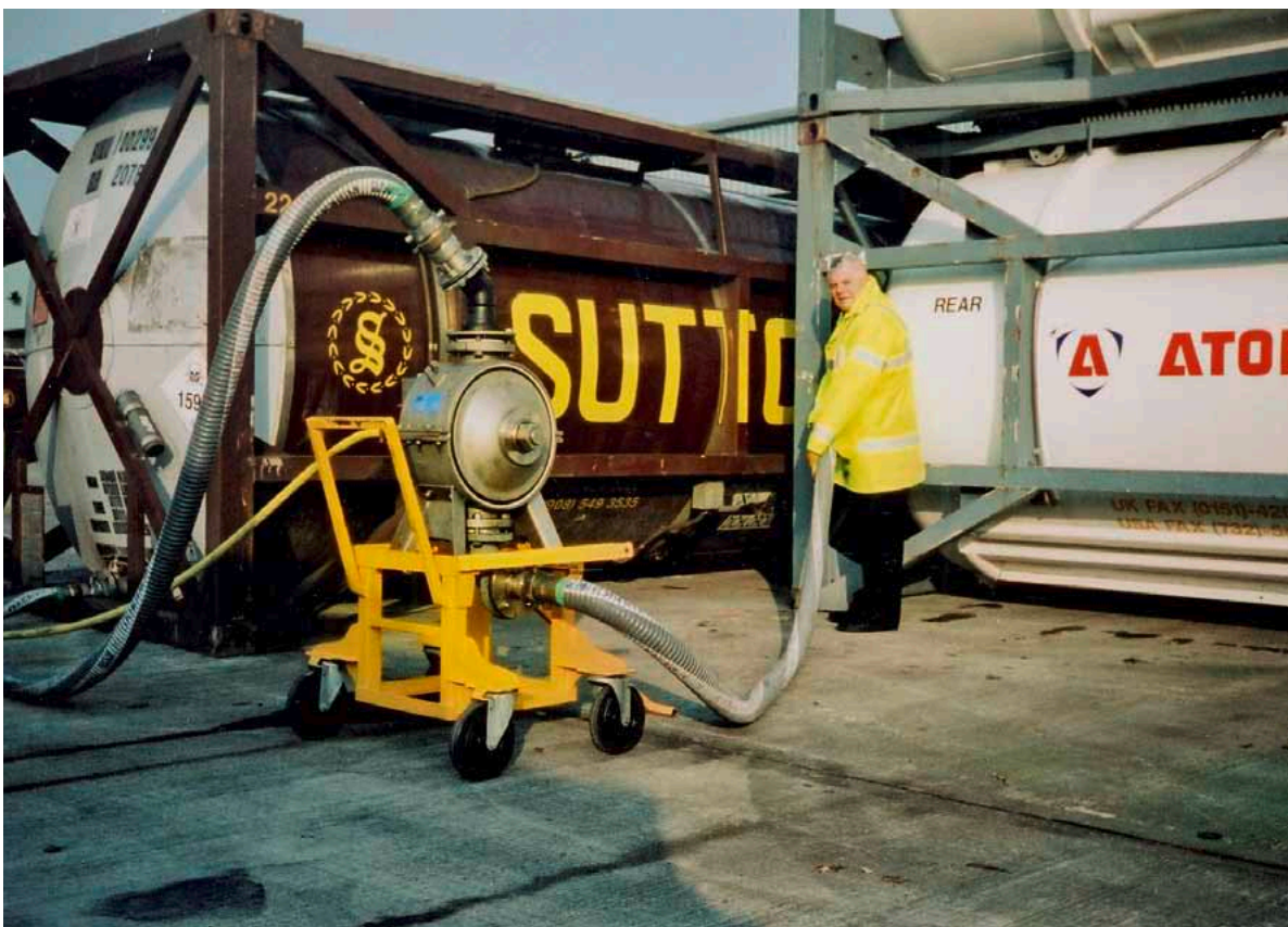
The pump handles different liquids i.e. diesel oil. It can empty a 30,000-litre tanker in less than two hours.
