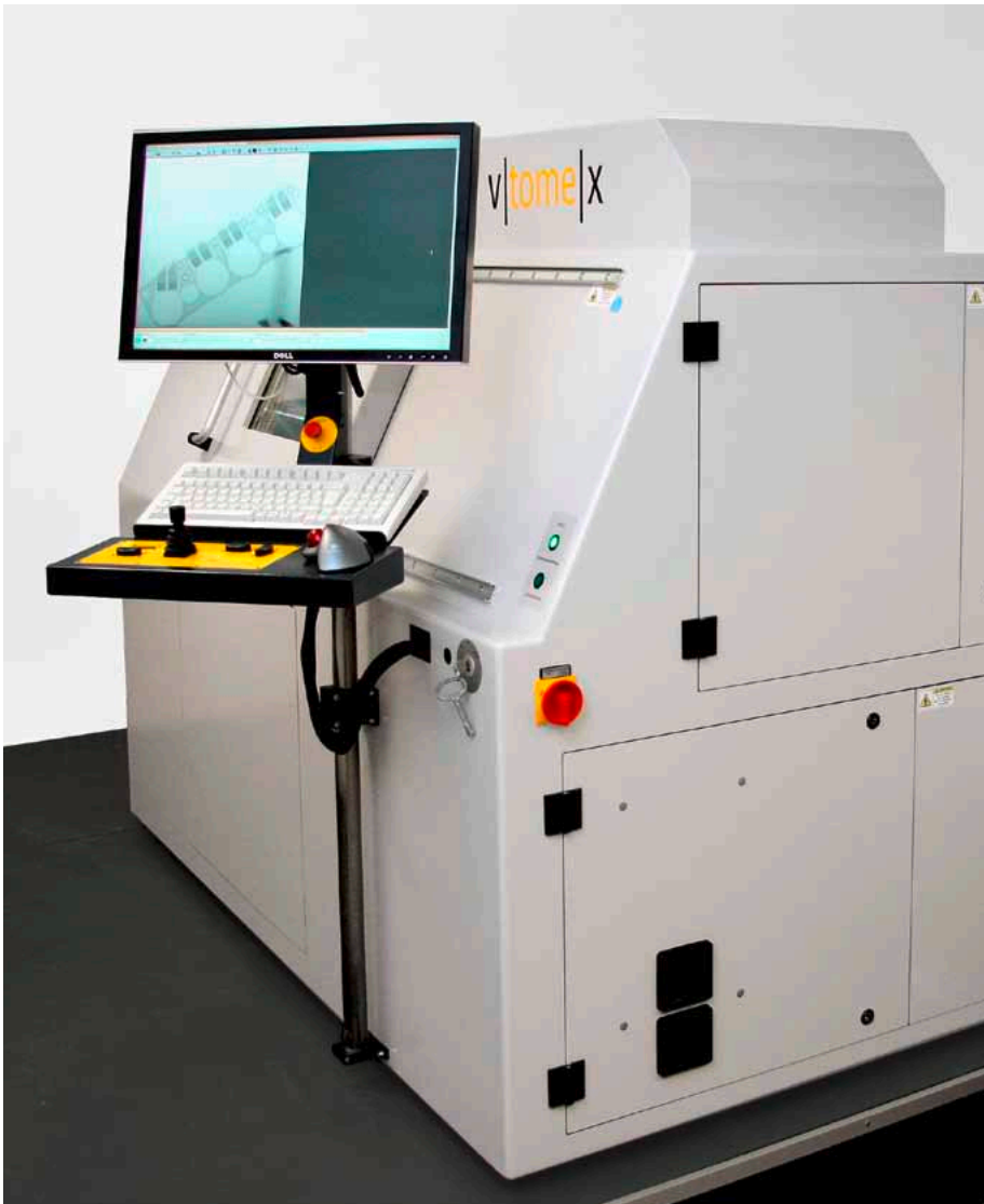
The CT scanner provides a three-dimensional view of what is inside a part.
